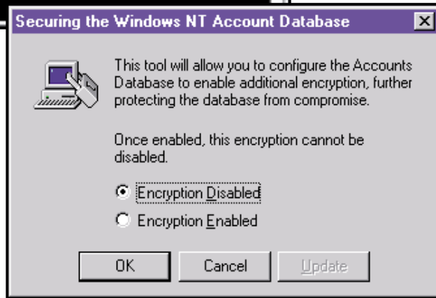
Securing your system with syskey makes it more difficult to defeat SAM security
